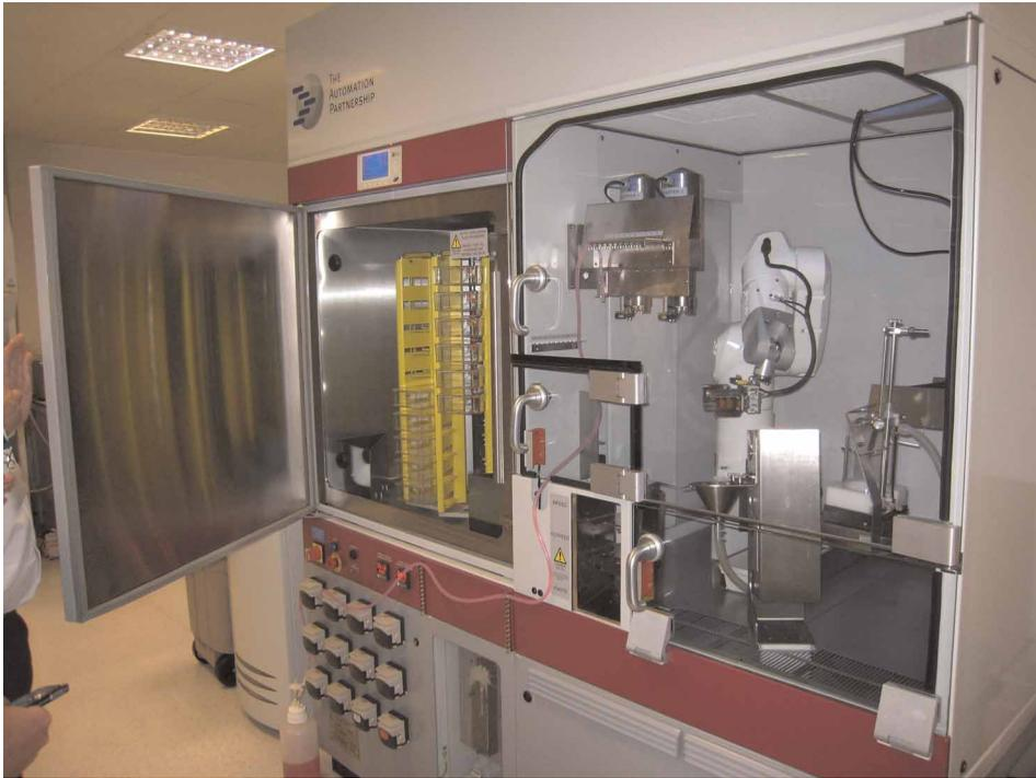
**Figure 2.** Working in close collaboration with The Automation Partnership (based in Nottingham), and with £1.85 M funding from the DTI, Intercytex has developed and process-validated a dedicated robotic system to enable commercial-scale production of living human cells. *Credit:* Sarah Franklin.
